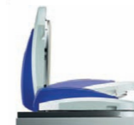
Lid closed, circumferential locking ring in lock position. The internal steam pressure presses the lip seal between lid and chamber.
